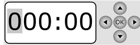
**Figure 1:** An example of 5-key user interface layout. Here the cursor is shown in the left-most position, and the display format is suitable for entering times, 0 minutes to 999:59 hours. Some 5-key interfaces omit the **OK** button as its use can be implied by the user performing any action with any non-arrow button.
