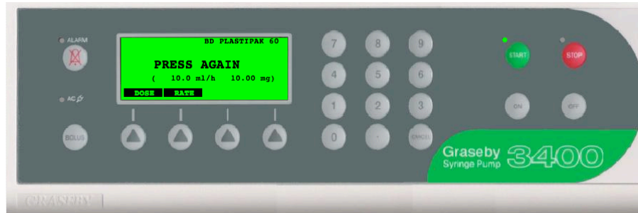
Fig. 1. Screen shot of the Graseby simulation in bolus mode, with the ‘start’ LED flashing, indicating that the device is infusing. The image was made by holding the Graseby 3400 over a scanner.
