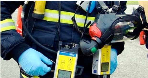
Figure 6. Mobile devices should be unambiguous when viewed from different directions. Here, seven segment radiation dosimeters hanging upside-down from the wearer’s belt can easily be read differently by a supervisor and by the wearer, who would lift them up to read them.
