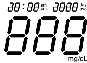
Figure 15. Part of the switch-on test display for the Roche Accu-Chek® Compact Plus [13] handheld blood glucometer (redrawn for this paper). The idea of the switch-on display is to confirm that all segments work; in fact two top left segments are never used (there is no physical need for them to show 12 or 24 hour times), so ironically the test display appears to be faulty because two segments are missing! Also notice the unusual high visibility decimal point (top right number), which is easy to implement in this sort of customised display.
