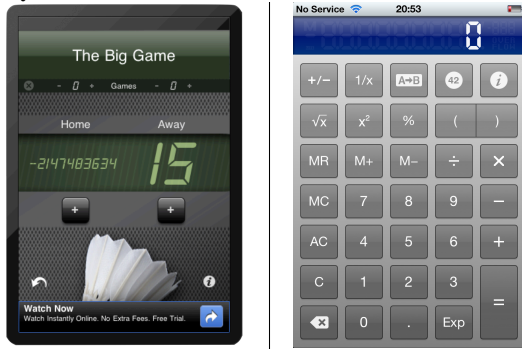
Figure 3. Screen shots of two iPhone applications. Seven segment digits are used to create a “retro” design feel despite the high resolution of the iPhone display — which has been used to render other high resolution text, including key legends.
