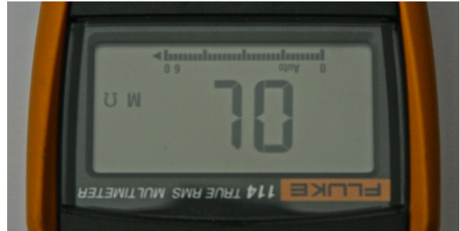
Figure 5. Digital multimeters are safety critical devices: mis-reading the display could lead to electrocution or other problems. Shown here is a Fluke 114 digital multimeter (a typical high-quality meter) upside-down. Is the (correctly functioning) display showing 70 or something else?
