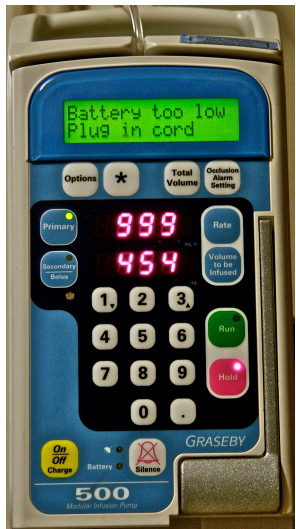
Figure 2. Graseby 500 infusion pump, illustrating typical number display design issues. (i) Numbers are shown using seven segment displays despite the available higher resolution dot matrix display. (ii) Units of displayed numbers are far too small to be read reliably. (iii) Number keys use a high resolution digit font that is different to the displayed digits. (iv) The digit keys 1 and 3 look like they have a decimal point; in fact, these digit buttons have two modes so they can also be used as arrow keys.
