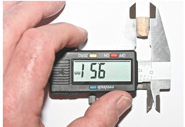
Figure 1. Digital calipers (used for measuring small items) shown held in the left hand, a situation that arises measuring awkward shapes or when the user is left handed. Here, the display might be read as 1.56 (cm?), misreading the space as a decimal point, when in fact it is displaying 9.51 mm. Note that the decimal point is very small and easy to misread.
