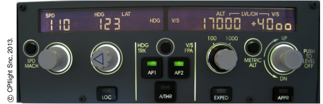
Figure 9. The Air Inter Flight 148 crash on 20 January 1992 had multiple causes. The excessive rate of descent may have been partly caused by the pilots inadvertently setting the autopilot in vertical speed mode instead of flight path angle mode (a double use of the rightmost number in the picture above). The pilots entered 33 intending a 3.3° descent angle, which the autopilot treated as a descent rate of 3,300 feet per minute (both would have been displayed as -33). Airbus later modified the display so vertical speed is displayed as a four-digit number (top right) and flight path angle as a two digit number with a decimal point, thus attempting to reduce possible confusion [1]. Interestingly, the Report of the Commission of Inquiry has a diagram [14, Figure 8] of the autopilot using hi-res digits.
