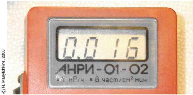
Figure 11. A handheld Russian radiation meter that misleadingly appears to be displaying two numbers, or perhaps a number and a mode, and it might even be misread as 0•16 if viewed from an oblique angle.
