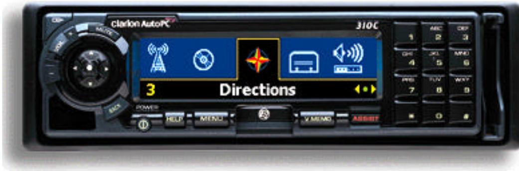
Figure 1: AutoPC: a car radio-sized PC (reproduced from Clarion's web site, <http://autopc.com/>, 1999).
