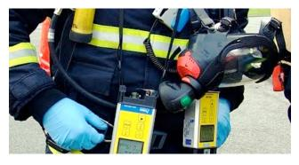
**Figure 3:** Mobile devices should be unambiguous when viewed from different directions. Here, seven segment radiation dosimeters hanging upside down from the wearer's belt can easily be read differently by a supervisor and by the wearer, who would lift them up to read them.
