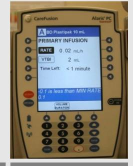
On this infusion pump, the rate is simultaneously shown as 0.02 mL/h and in an error warning as -0.1. What does the log say?
