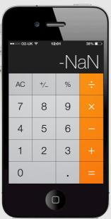
NaN ("not a number") shows the calculator has made an internal error. Critically, if the user continues the error message disappears and incorrect results will be displayed. (In the middle of a calculation, users are more likely to be looking at the keypad than at the display, so transient error messages won't be seen.)
