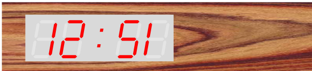
Figure 7. A clock showing 12:51 or 15:21? Displays like these are small enough to be put in the bodies of pens, so there is no natural up or down orientation, which is particularly problematic for left-handers.
