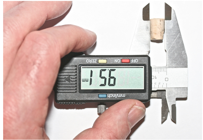
Figure 1. Digital calipers (used for measuring small items) shown held in the left hand, a situation that arises measuring awkward shapes or when the user is left handed. Here, the display might be read as 1.56 (cm?), misreading the space as a decimal point, when in fact it is displaying 9.51 mm. Note that the decimal point is very small and easy to misread.
