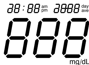
Figure 15. Part of the switch-on test display for the Roche Accu-Chek® Compact Plus [13] handheld blood glucometer (redrawn for this paper). The idea of the switch-on display is to confirm all segments work; in fact the top left segment is never needed for 24 hour times (so there is no physical need for one), so ironically the display appears to be faulty! Notice the high visibility decimal point (top right number), which is easy to implement in this sort of customised display.
