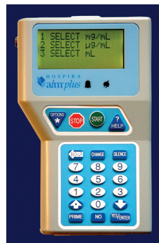
► Figure 1. The infusion pump used in the fluorouracil incident. The pump is small and gives the patient full mobility during the treatment. Here, the nurse needs to enter mL per hour but has to use Option 3, which is apparently asking for mL! Note that the up arrow key doubles as the decimal point.
