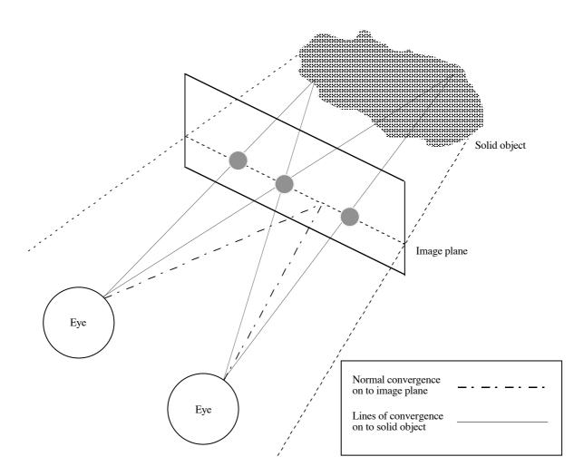
Figure 1 Simulating a solid object on a 2D image plane
