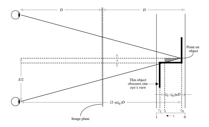
Figure 4 Geometry for hidden surface removal
